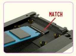
Insert M.2 (M Key & Connector matches in the same way)
