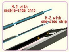
Check M.2 SSD type\* for suitable thermal pad
