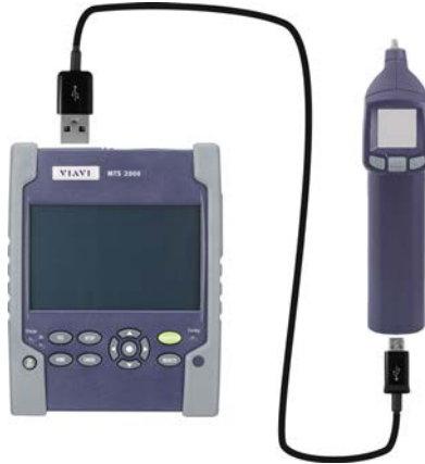
Figure 17 USB connection of the FiberChek probe
