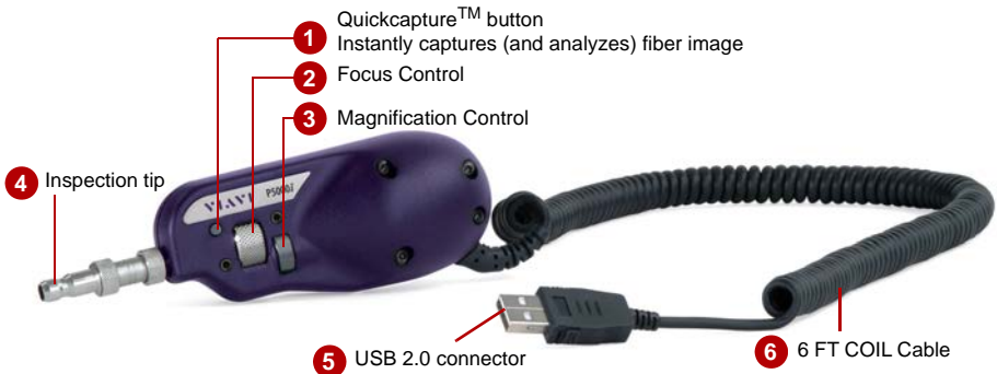
Figure 14 P5000i Probe components
