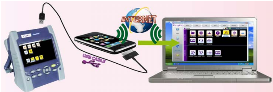
Figure 45 USB connection through Smartphone
