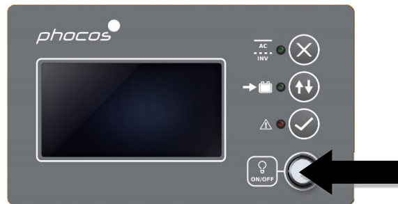
Fig. 11: Load output ON/OFF button location
