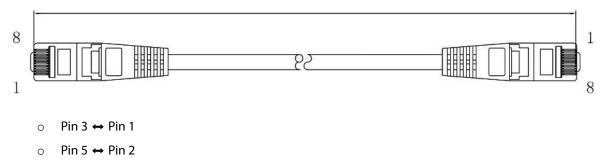
This way 4 pins (number 1, 2, 3 and 5) are connected on each side of the cable. It is not relevant which way the cable is oriented between the battery and PSW-H unit.
