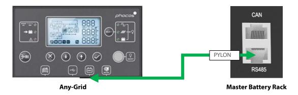
For systems with multiple Any-Grids, this connection (marked green) can be made with any of the inverters, but only a single unit. Remember, all Any-Grids in a synchronised system must be connected to a single battery bank as shown here for a system with 4 Any-Grids in parallel:
