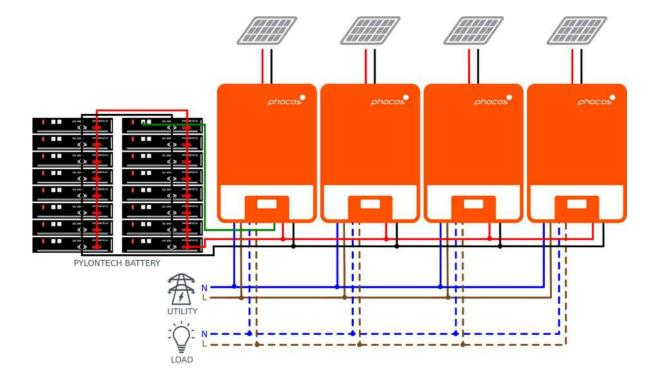
6. Ensure the battery racks are wired as outlined in the Pylontech battery manual. Turn on each of the battery racks with the power button and ensure the LED near the power button is green for all battery racks:
