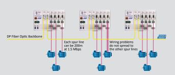
Long spur lines to instruments and the possibility to remove/insert them during operation. Short circuit protection on each spur line is automatically provided.
