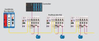
Creating a fiber optic backbone increases network reliability and network overview. It is also possible to mix ProfiHubs with ComBricks.
