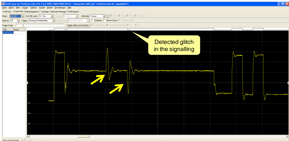
Fig. 46 - EMC/EMI disturbances
