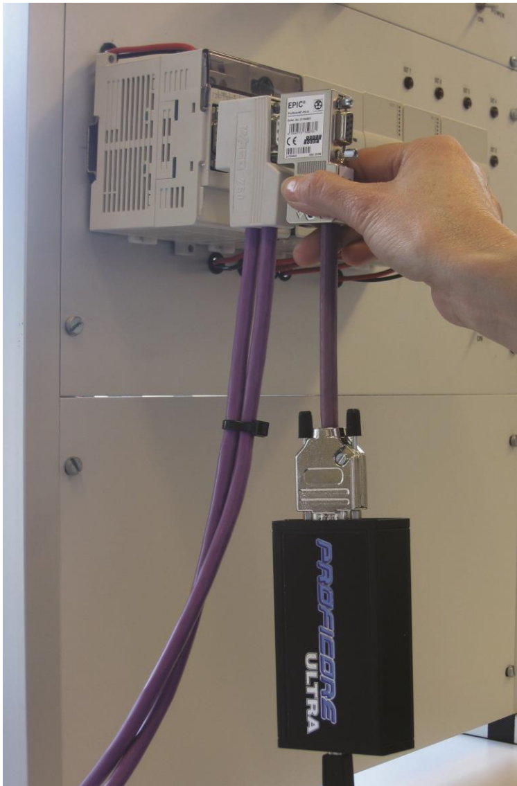
Fig. 10 - Attaching the ProfiCore to a DP installation
