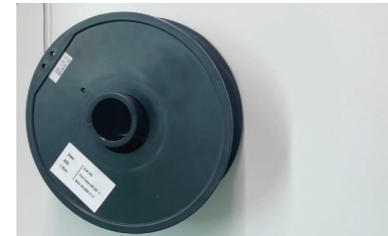
5 1. Install the spool holder. 2. Slide the filament spool onto the holder.
