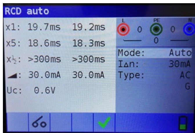
Figure 5-27: Step 8 RCD autotest results
