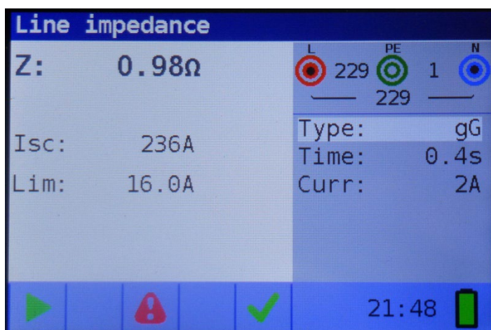
Figure 5-37: Example of line impedance measurement results
