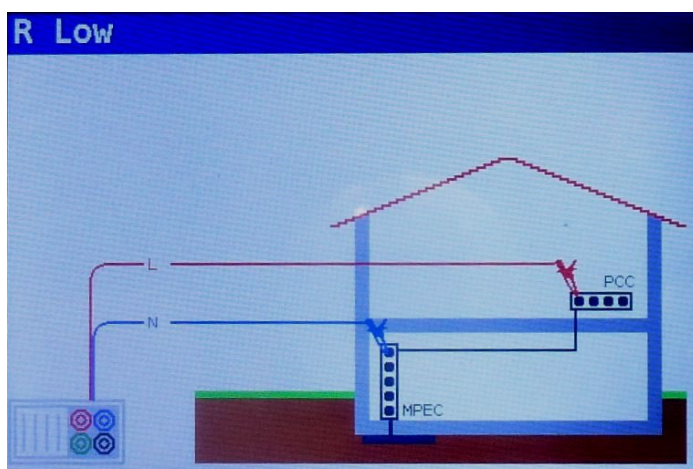
Figure 5-6: Connection of universal test cable
