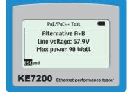
If this voltage is below the standard value, the KE7200 will switch the load back until the voltage is within the normal range again.
