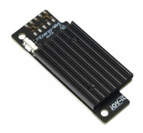
With the PiEnergy-Mini, you can operate your Raspberry Pi with a voltage of 6 to 36 V DC. You can use the button integrated on the board to both power up and power down your Raspberry Pi. Communication with the Raspberry Pi is via GPIO4, but this connection can also be cut by removing a resistor to use the pin freely. Thanks to the ultra-flat design, it can also be used in many housings. The pin header is included and not soldered on to keep the design even flatter.
