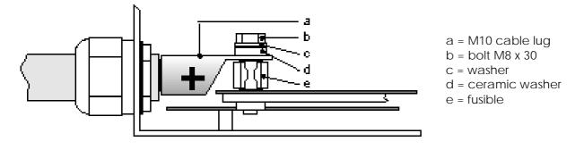
Be careful with the orientation of the ceramic washer. There is a small lip on one side which must fit into the cable lug's hole.
