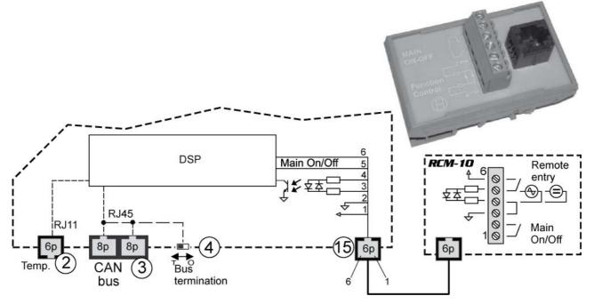
It is also possible to access to these functions by a direct cabling on the RCM-10 plug of the device (15) as per the opposite pictures.
