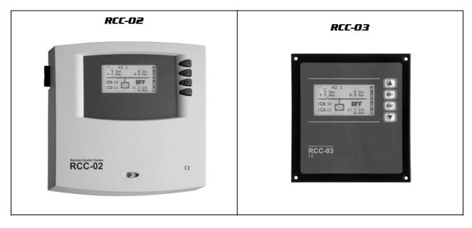
The features of the RCC-02 and the RCC-03 are the same. They only differ in their external appearance. The RCC-02 is designed for wall mounting, whereas the RCC-03 is designed as a board device.
