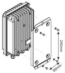
An external cooling fan (ECF-01) can be installed before or after the equipment has been mounted on the wall in order to improve its performances.
