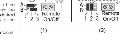
Contact by a voltage (max. 60V eff. / 30mA): the jumpers are set as in (2) A1-B1 and A2-B2.
