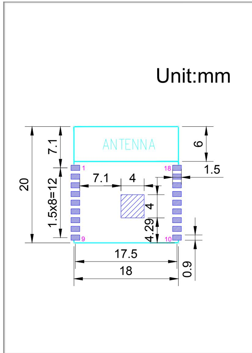
Figure 7-1. Recommended PCB Land Pattern of ESP-WROOM-02
