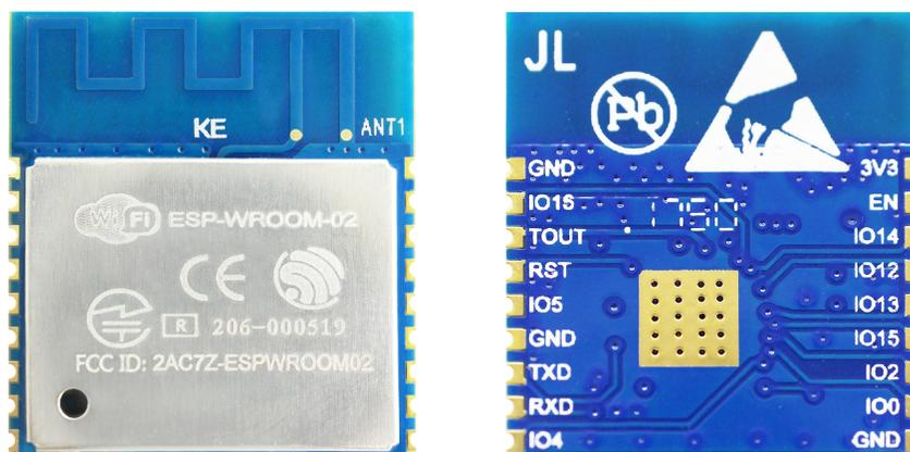
Figure 1-1. ESP-WROOM-02 Module
