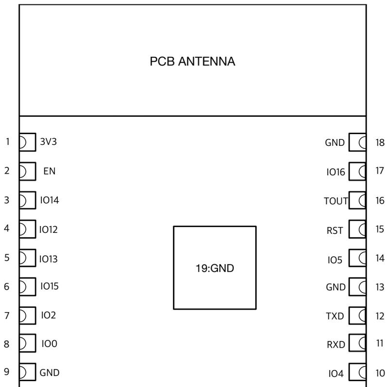
Figure 2-1. ESP-WROOM-02 Pin Layout (Top View)
