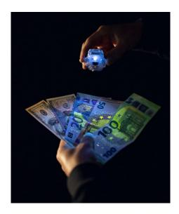
Ultraviolet light with 365 nm wavelength is for verification of currency and passports authenticity, revealing household stains, detecting leaks
