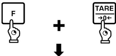
⇒ Press [**F**]- key and [**TARE/ZERO**] key simultaneously for about 2 seconds.
