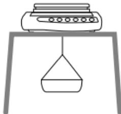
⇒ Attach empty immersion basket to hooks for underfloor weighing.
