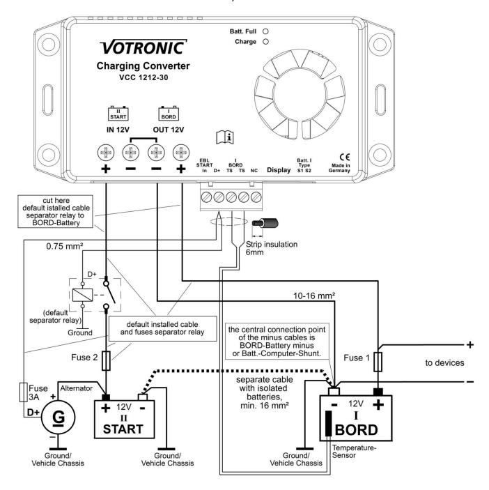
Note: During external mains charging, the recharging branch of the VCC 1212-30 for charging/trickle charging of the STARTER battery from the BOARD battery is not active. (The cutoff relay is switched off.)
