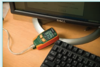
USB connector easily plugs into a computer for data analysis of Temperature and Humidity
