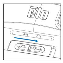
Lift-up the battery, then slide up away from the compartment.
