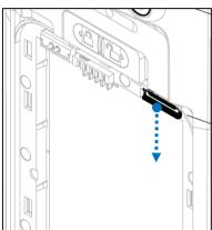
• Place the Micro SD and/or the Nano Sim card into the carrier with contact side face down.
