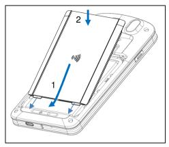
While pressing down slide the battery lock to the left (into the locked position) to secure the battery.
