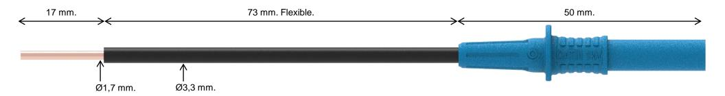
Stripped 2,50 mm<sup>2</sup> (approx. AWG13) rigid copper wire to connect to screw terminal blocks.
