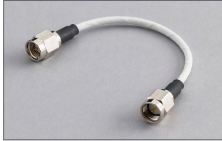
CA-451A: 10.8 cm (4.25 in) RG188 coax cable terminated with an SMA male plug on each end, 50 \Omega impedance.
