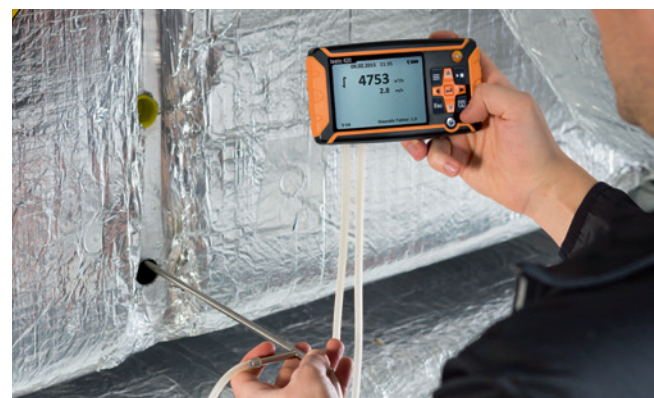
Removable instrument allows Pitot tube measurements in ducts (Pitot tube available separately)
