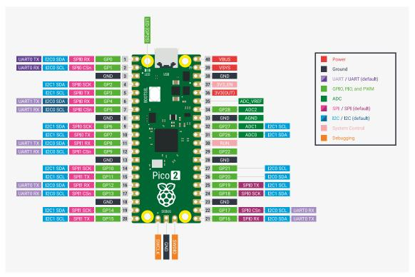
Pico 2 uses an on-board buck-boost SMPS which is able to generate the required 3.3 V (to power RP2350 and external circuitry) from a wide range of input voltages (1.8 to 5.5 V). This allows significant flexibility in powering the unit from various sources such as a single Lithium-ion cell, or 3× AA cells in series. Battery chargers can also be very easily integrated with the Pico 2 powerchain.
