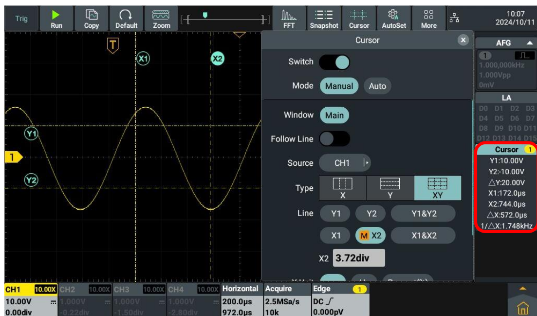
Figure 5-9:Time &Voltage Cursor Measurement
