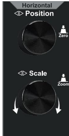
Figure 5-3: Horizontal control area
