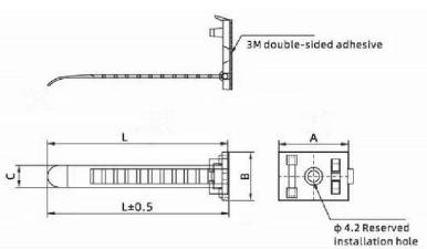
**Technical Data:** Material: Polyamide (PA66) • Color: Black or White • Length of Clamping-Strap (L): 66 ... 94 mm • Adhesive tape: 3M quality adhesive tape • Content: 50 pcs. • Temperature range: -20 ... +80 °C.
