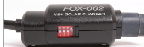
Switch for selecting charging characteristics
