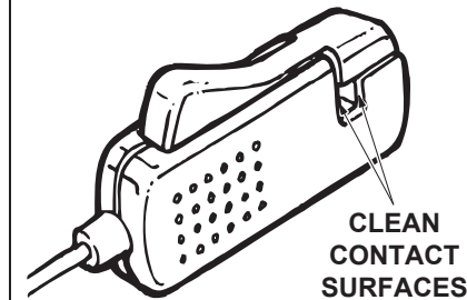
Fig. 6. Cleaning the Inductive Pickup Clip
