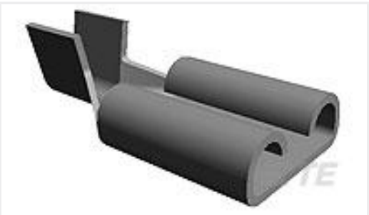
TE Part #42399-1 110 FASTON REC 20-18 AWG TPBR
