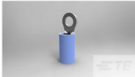
TE Part #36157 TERMINAL,PIDG R 16-14 6
