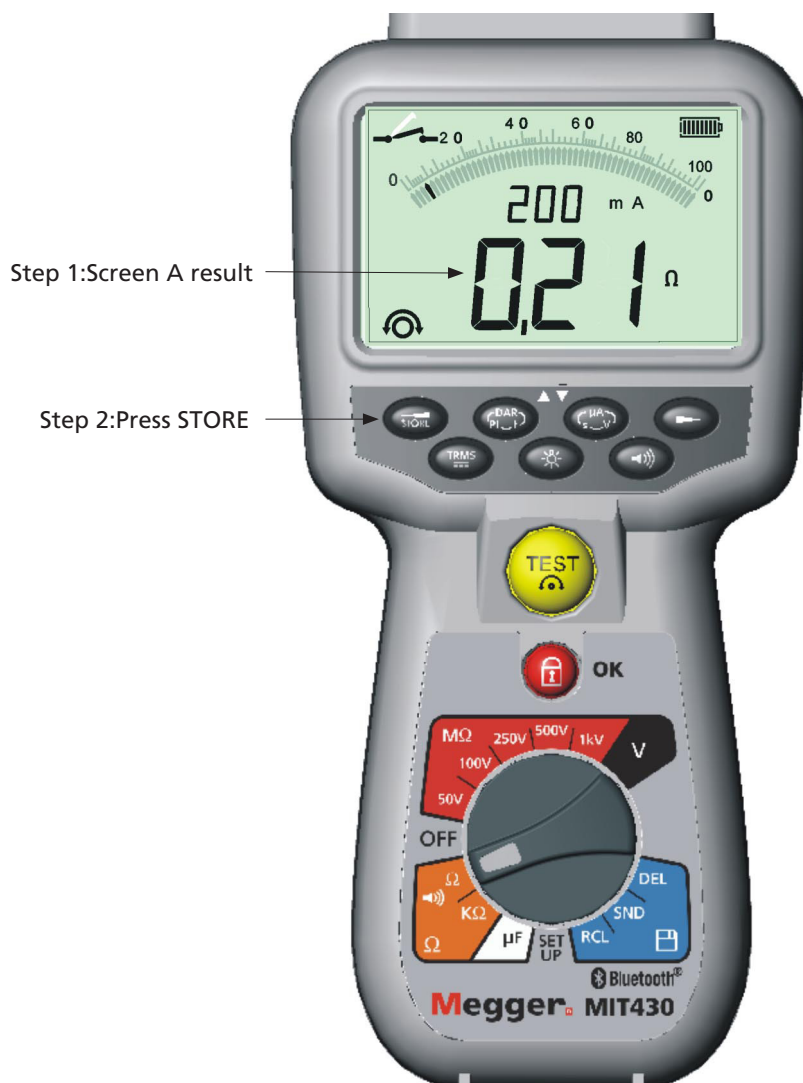
Figure 13 Test results storage
