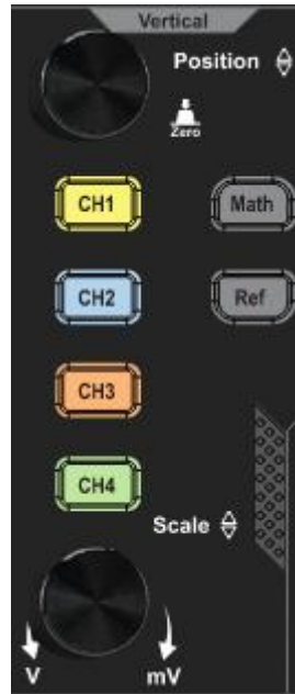
Figure 5-3: Vertical control area
