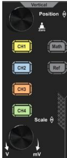
Figure 5-3: Vertical control area
