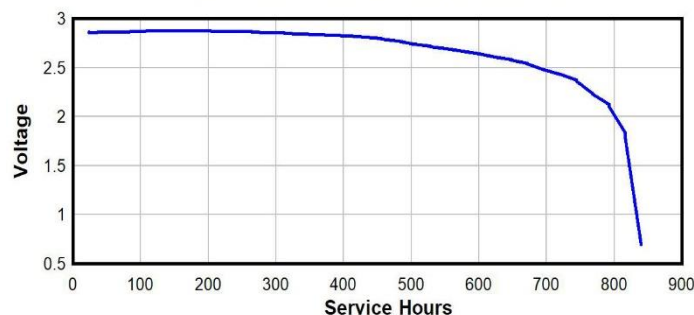
Low Load Pulse Testing 300mA Pulse with 2mA Background to 1.8V
