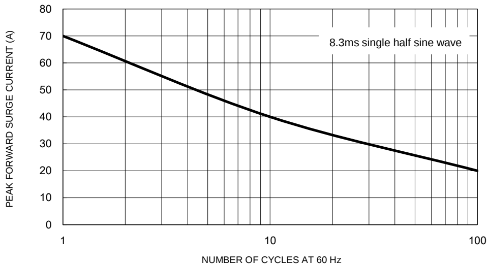
Fig.11 Maximum Non-Repetitive Forward Surge Current
