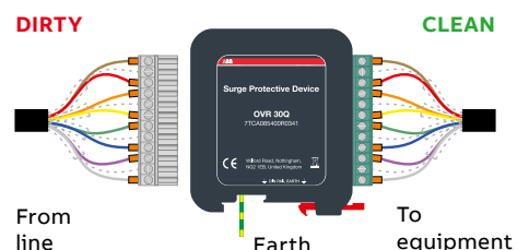
OVR 06Q, OVR 15Q, OVR 30Q, OVR 50Q and OVR 110Q installed in series (in-line)
