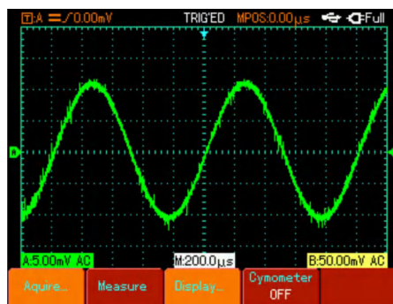
Figure 2-20 Waveform without average sampling
