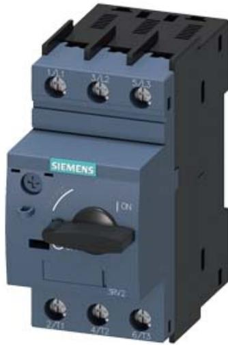
INTERRUPTOR AUT. TAM. S00, P/ PROTEC. MOTORES, CLASE 10, DISP. A 10...16A, DISP. N 208A, BORNES DE TORNILLO, PODER DE CORTE ESTANDAR
