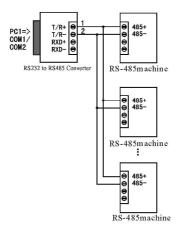
3. half-duplex communication connect between interface converter
