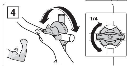
**EN** 1. Fit the knob as in the diagram. 2. Tighten the screw until it is no longer possible to undo the knob by hand. **3-4.** Loosen the screw  $\frac{1}{2}$  a turn at a time until it is possible to turn the knob by hand (**the knob should not move easily when it is loosened**).
