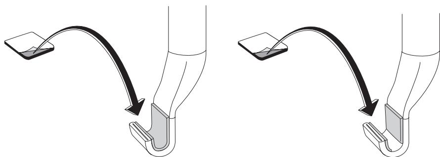
**EN** Check that the hooks remain free when shut. If the lower hooks strike the bumper, the rubber protector can be split and fitted on the sides of the lower hooks.
