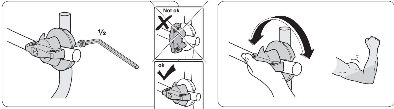
**EN** **Check the tension.** After a period of use, it may be necessary to check the tension in the knob. Tighten the hexagonal screw half a turn and check that there is greater resistance in the knob when you turn it. **NOTE:** The knob should always be in the tensioned setting.
