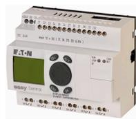
Automate compact, 24V DC, 12 entr. TOR (dont 4 entr. analog.), 6 sort.TOR (R), CAN, afficheur
