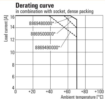
\* For full continuous current (16 A), socket connections 11-21, 12-22 and 14-24 must be bridged.
