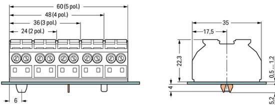
Dimensions (in mm) for chassis-mount terminal strips
