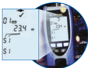
Test câblage coaxial
