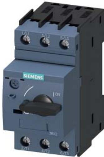
DISJONCTEUR TAILLE S00, POUR PROTECT. MOTEUR, CLASS 10, DECL.A 10...16A, DECL.N 208A, BORNES A VIS, POUVOIR DE COUPURE STANDARD
