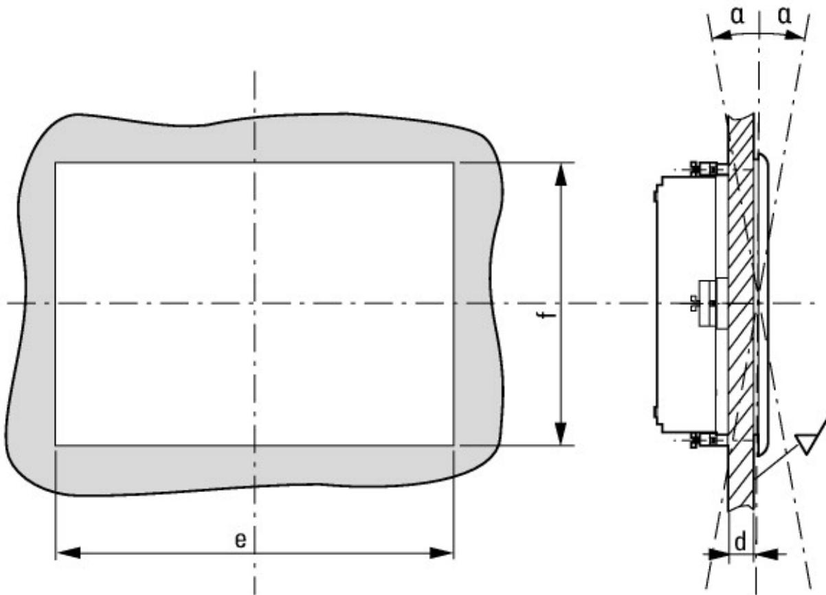
$2 \text{ mm} \leq d \leq 5 \text{ mm}, e = 255,5 \text{ mm}, f = 160,5 \text{ mm}, \# = 45^\circ$
