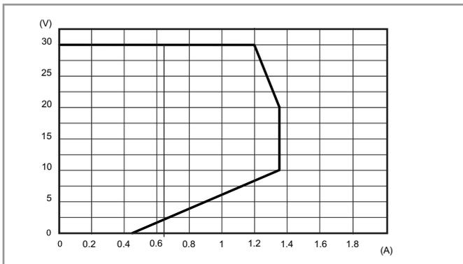
Diagramme de surcharge, conforme KNX
