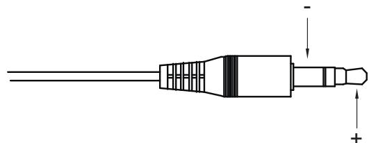
**Note:** check the technical documentation of your equipment to decide whether the IR module of the IR control 10 XTRA can be connected directly. Most IR cables use a 3.5mm mono jack connector where the tip is used for the “IR Data” and the sleeve for “GND”.
