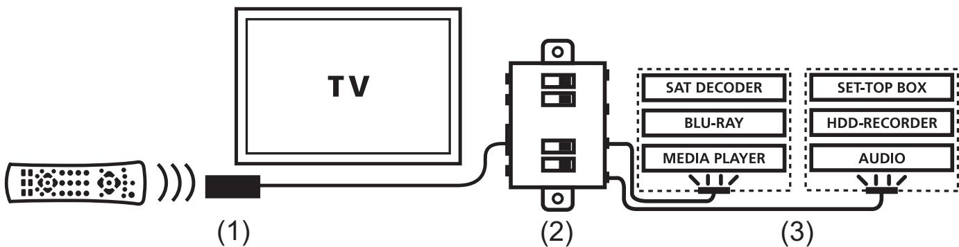
The IR Control 10 XTRA™ is made up of three main components;
