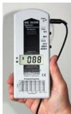
Insert the plug of the enclosed grounding cable into the dedicated socket of the meter  $\perp$  and run the cable along the side of the case to the back (see picture). Make sure that neither the grounding cable nor the user's hand is in the front of the meter (falsifies the reading!).
