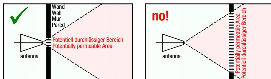
For the definition and installation of shielding measures as well as surveying their effect, professional advice is recommendable. Anyway, the area covered by shielding material should be much larger than the leak itself.
