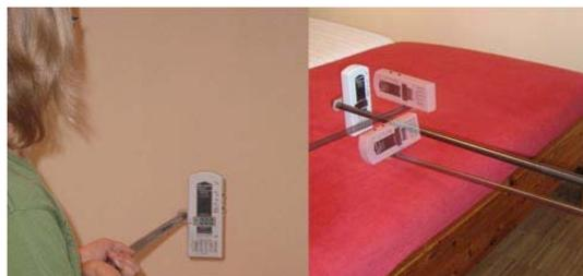
hertz Solutions), three measurements in the three dimensional axes XYZ (see figure on the left) and the vectorial addition<sup>2</sup> of their results.
