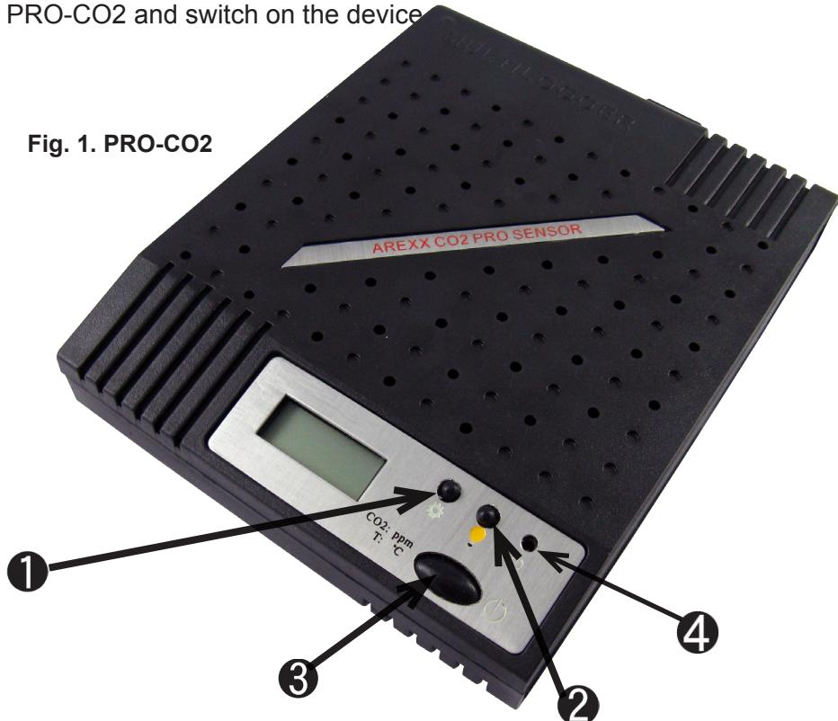
After switching on the device the LED (4) will light up and the sensor immediately transmits its first sensor data.
