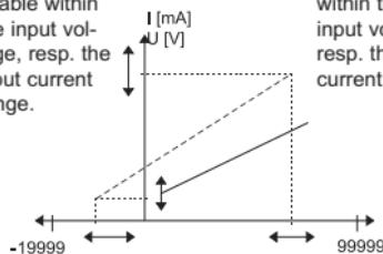
Minimum input voltage or minimum input current freely positionable within the input voltage, resp. the input current range.
