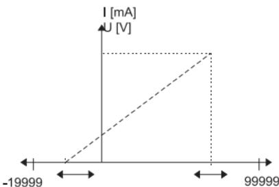
The selected measuring range is 0...20 mA. Assign the value 0 to the lowest input signal and 10 to the highest. To display the sum in tons, set a factor of 0.001.
