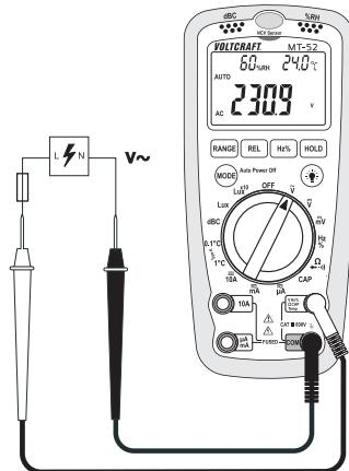
The mV-AC measuring range can only be selected via manual measuring range selection ("RANGE" button).
